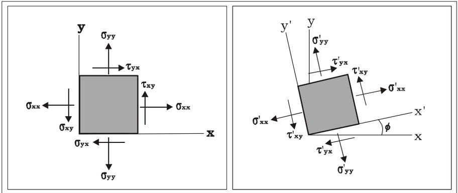
The relationship between the original state of stresses ( $\sigma_{xx}$ ,  $\sigma_{yy}$ ,  $\tau_{xy}$ ,  $\tau_{yx}$ ) and the state of stress when the axes are rotated counterclockwise by  $\phi$  ( $\sigma'_{xx}$ ,  $\sigma'_{yy}$ ,  $\tau'_{xy}$ ,  $\tau'_{yx}$ ), can be represented graphically by the construct shown in the figure below.
