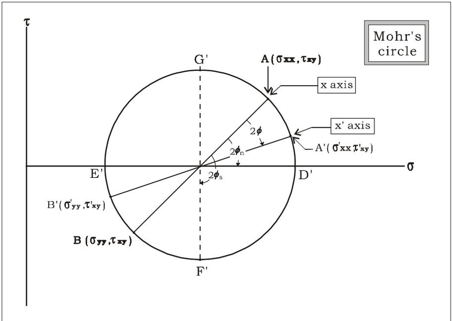
The stress condition for which the shear stress,  $\tau'_{xy}$  is zero, indicated by segment  $D'E'$ , produces the so-called *principal stresses*,  $\sigma_{xx}^P$  (at point  $D'$ ) and  $\sigma_{yy}^P$  (at point  $E'$ ). To obtain the principal stresses you need to rotate the coordinate system  $x'-y'$  by an angle  $\phi_n$ , counterclockwise, with respect to the system  $x$ - $y$ . In Mohr's circle, the angle between segments  $AC$  and  $D'C$  measures  $2\phi_n$ .
