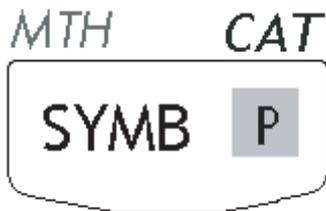
Notice that the color and the position of the labels in the key, namely, **SYMB**, *MTH*, *CAT* and **P**, indicate which is the main function (**SYMB**), and which of
