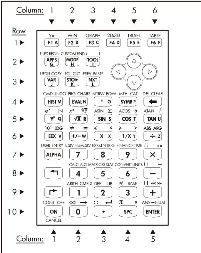
The figure shows 10 rows of keys combined with 3, 5, or 6 columns. Row 1 has 6 keys, rows 2 and 3 have 3 keys each, and rows 4 through 10 have 5 keys each. There are 4 arrow keys located on the right-hand side of the keyboard in the space occupied by rows 2 and 3.
