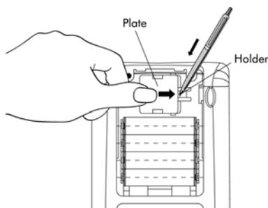
b. Insert a new CR2032 lithium battery. Make sure its positive (+) side is facing up.
