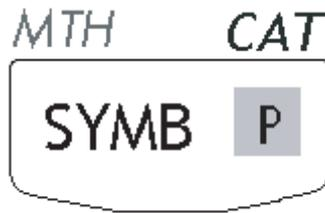
Notice that the color and the position of the labels in the key, namely, **SYMB**, **MTH**, **CAT** and **P**, indicate which is the main function (**SYMB**), and which of the other three functions is associated with the left-shift **←** (**MTH**), right-shift **→** (**CAT**), and **ALPHA** (**P**) keys.
