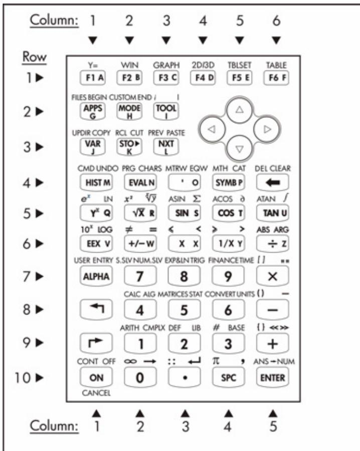
The figure shows 10 rows of keys combined with 3, 5, or 6 columns. Row 1 has 6 keys, rows 2 and 3 have 3 keys each, and rows 4 through 10 have 5 keys each. There are 4 arrow keys located on the right-hand side of the keyboard in the space occupied by rows 2 and 3. Each key has three, four, or
