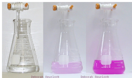
Fig 2 – Colors observed during a titration – don't go too far.
