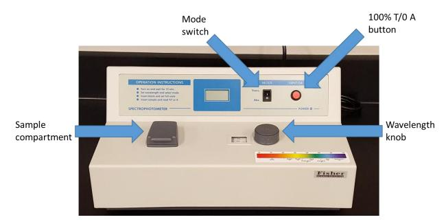
**Collect background** – This corrects for the absorption by the cuvette and solvent. It needs to be done for each set of samples. Background collection can be done in either transmittance or absorbance mode.
