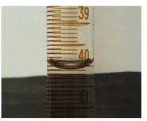
zone of white. Note in the photo at the left that the apparent level of the meniscus is different from that on the right. Since placing the black streak just under the meniscus is more repeatable than at some variable distance, the close placement is recommended.
