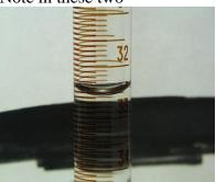
The use of a buret card and a line of sight perpendicular to the buret column are techniques which must be adopted to achieve maximum precision. Note the final photograph in which the level of the meniscus bottom can be determined to within  $\pm 0.01$  mL. What reading would you report for this buret volume?
