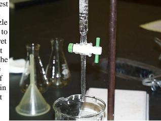
bubbles out. If that doesn't work, two other methods can be used. The first is to use some chaotic suction. The student on the left has first rinsed then filled her buret with titrant.
