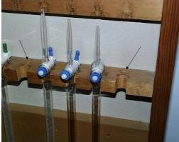
arrows pointing to the holes into which one "ear" of the petcock valve is placed. Placing the buret in the cabinet this way assures that the buret won't fall out when the cabinet is opened.
