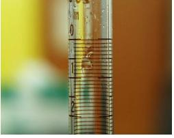
A 50 mL buret can be read to  $\pm 0.01$  mL, but in order to be able to interpolate to the last digit, the perpendicular line of sight must be followed with meticulous care. Note in these two
