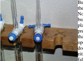
But get a load of these two pictures. Notice how the burets have been placed precariously so that just a quick opening of the door will allow either to slip out, fall on the floor
