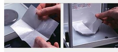
Place creased, small weighing paper on the balance pan.
