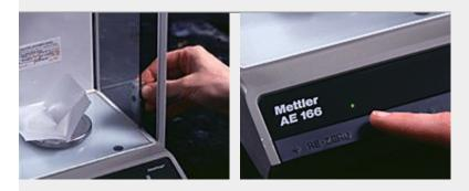
Close the sliding glass doors. Wait for the green dot on the left to go out. This is the stability indicator light, indicating that the weight is stable.
