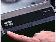
Press the control bar to cancel out the weight of the container or paper. The display will again read 0.0000.
