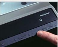
Turn the balance on by pressing the control bar. The display lights up for several seconds, then resets to 0.0000.
