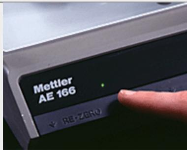
Close the sliding glass doors. Wait for the green dot on the left to go out. This is the stability indicator light, indicating that the weight is stable.
