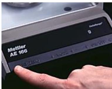
Press the control bar to cancel out the weight of the container or paper. The display will again read 0.0000.
