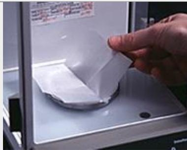
Place creased, small weighing paper on the balance pan.
