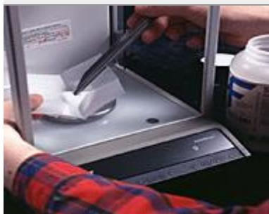
Carefully add the substance to be weighed up to the desired mass. Do not attempt to reach a particular mass *exactly*.
