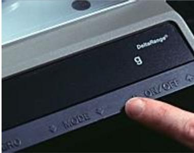
Turn the balance on by pressing the control bar. The display lights up for several seconds, then resets to 0.0000.
