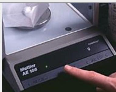
Before recording the mass, close the glass doors and wait until the stability detector lamp goes out. Record mass of solid.
