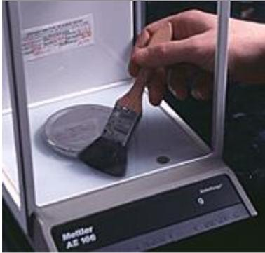
Use the brush provided to clean spills in the weighing chamber. Discard any disposable tare containers, weighing paper, or Kimwipes in the nearest wastebasket.
