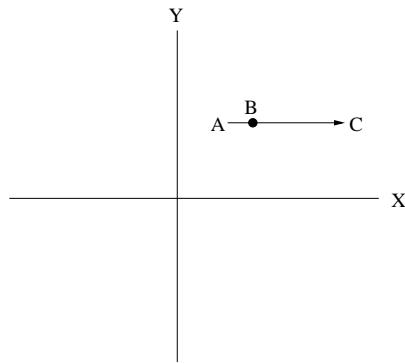
13. The arrow above has endpoints **A** and **C** defined by points with coordinates  $(3,3,0)$  and  $(9,3,0)$  respectively. In addition, the rotation point **B** is defined by the coordinates  $(5,3,0)$ . You are viewing the figure from the positive Z-axis.
