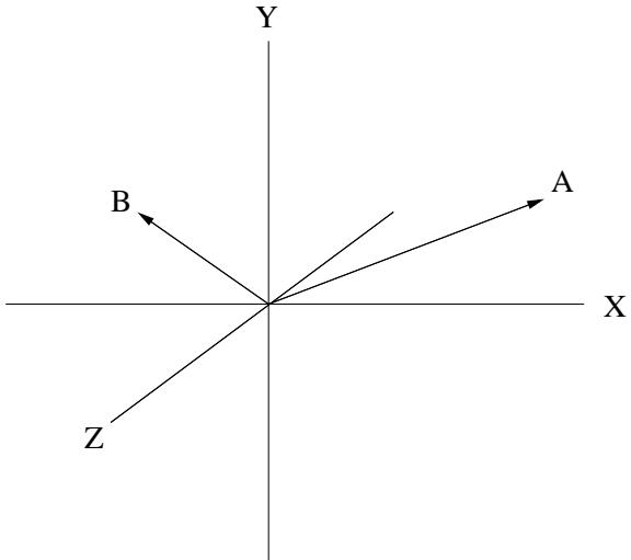
15. The diagram above shows two vectors starting at the origin. Vector **A** terminates at the point (8,3,4). Vector **B** terminates at the point (-4,3,3).
